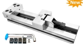
APEX CODE 794 High Precision Modular Vice With Parallel Top Jaws Accuracy 0.02 MM Hardness 57-62 HRC
